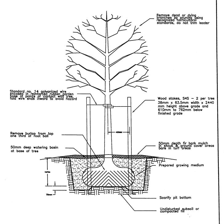
Note: Place tree & backfill 50mm above grade to allow for settlement
